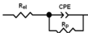
Fig. 7. ECA for the interpretation of electrochemical impedance spectroscopy data of barrier-coated metal
