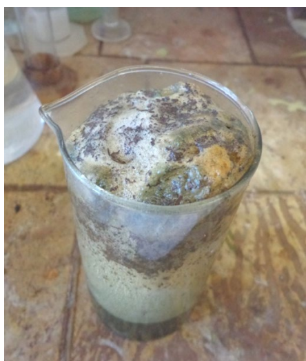
Fig. 4. Hydrogen release process across the entire surface of the magnesium turning Fig. 5. Precipitate after reaction with turning
