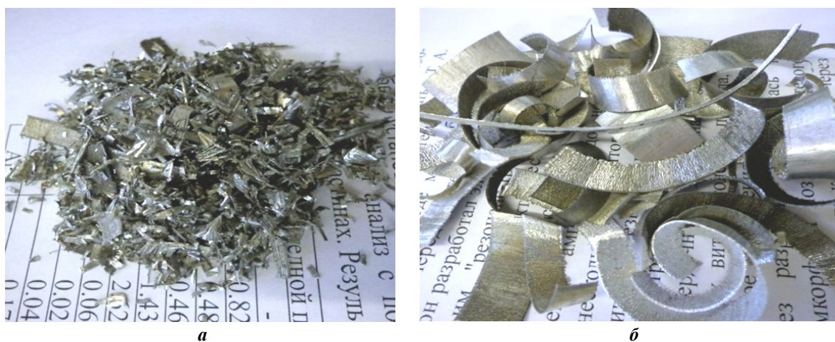
Fig. 3. Magnesium turnings: a – wool; b – heavy
