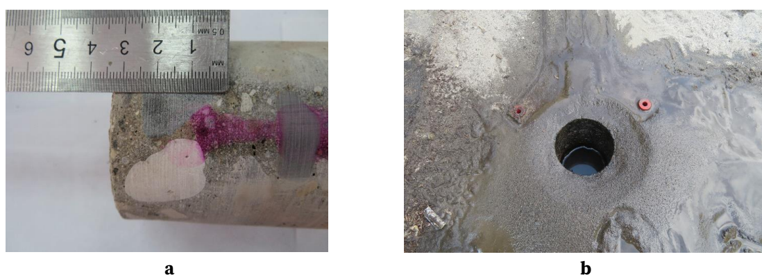
Fig. 2. Phenolphthalein indicator for carbonization conducted on a selected core sample (a) and the diamond drill site selected for the core sample (b)
