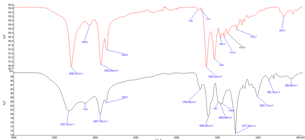
Fig. 4. IR spectra of the polyamide (lower graph) and the degraded polyamide yarns (upper graph)
